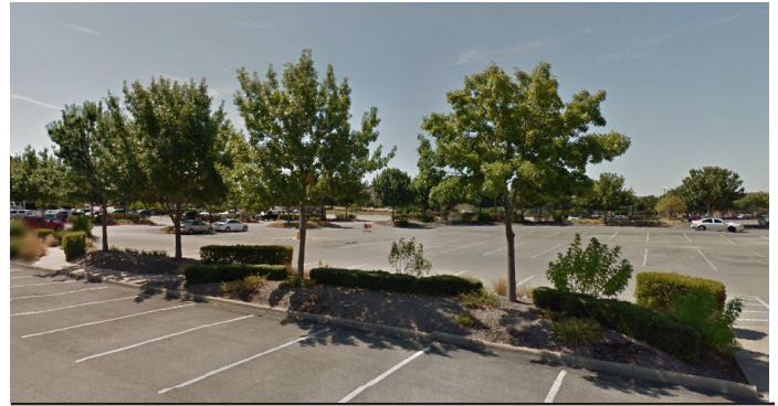
Good Example: Large soil volume, shade trees are clustered, soil is higher where the trees are placed to prevent people walking through and compacting the soil. The trees have more soil volume and are not competing with turf or getting damaged by mechanical equipment.
