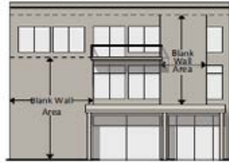
FIGURE 4.19 BLANK WALL AREA
