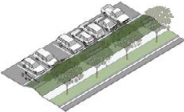
FIGURE 7.10 LANDSCAPING STRIP WITH BERM
