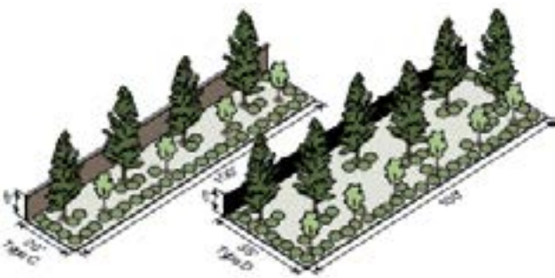
FIGURE 7.14 TYPE C AND D PROTECTIVE YARDS
