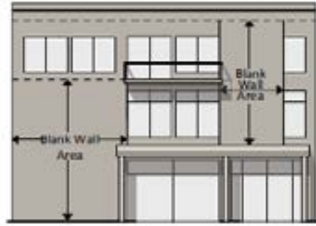
FIGURE 4.19 BLANK WALL AREA
