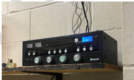
The pool amplifier is a consumer grade product and does not provide sufficient power for the system.
