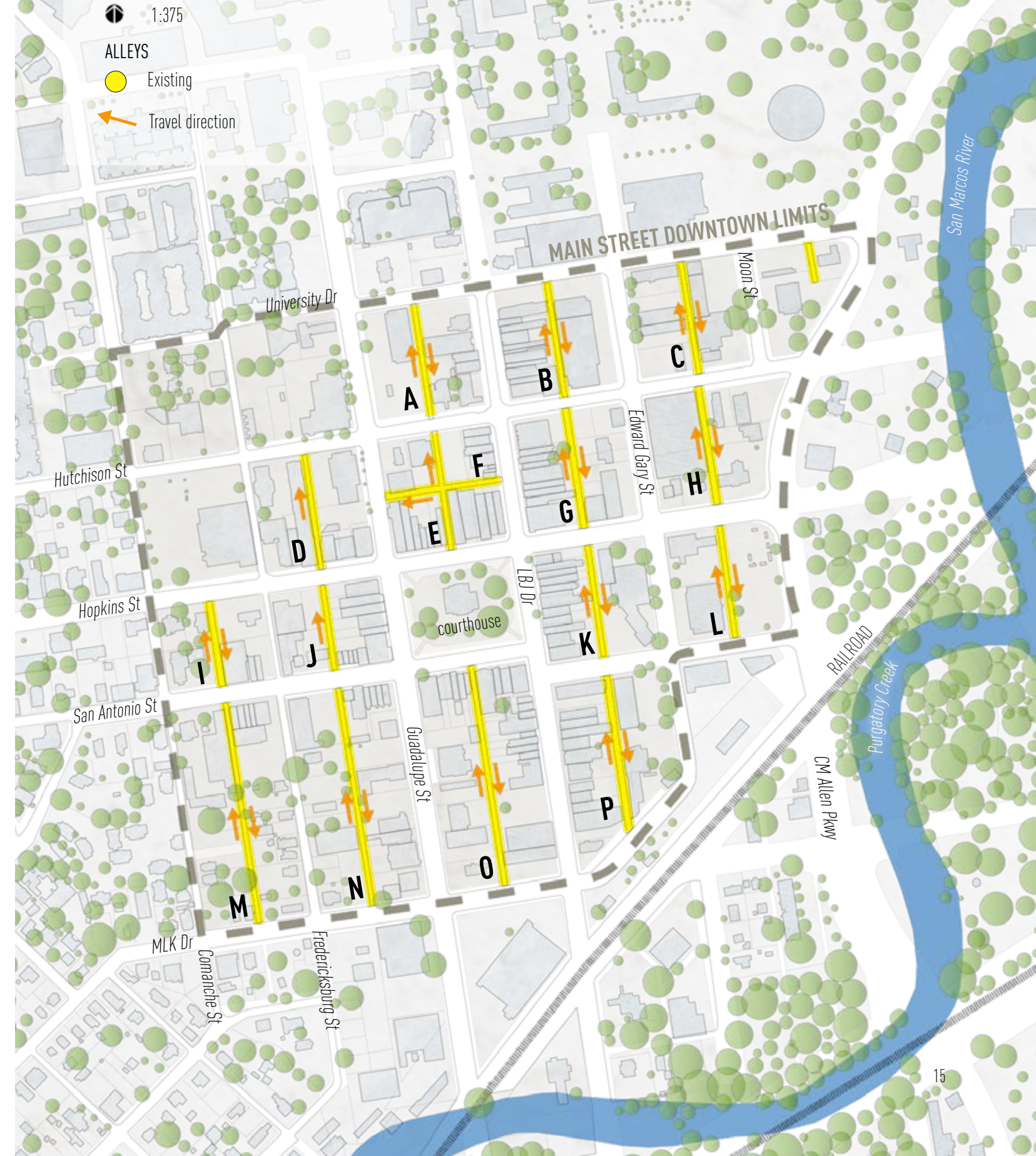
FIG. 14 DOWNTOWN SAN MARCOS ALLEY INVENTORY
