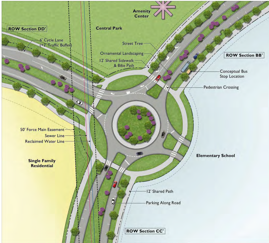
Illustration 26: Roundabout Plan View and Typical Future Bus Stop Plan (UPDATED)
