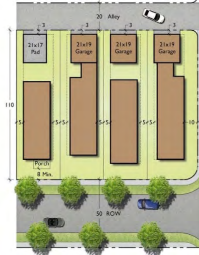
Illustration 35: Typical Lot Layouts SF-4.5 – SF Alley Loaded 32' and SF Alley Loaded 40'
