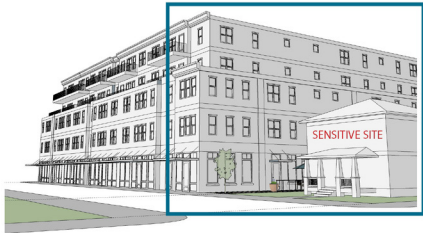
Recommendation Option B: This model illustrates the second option, where part of the building steps back away from the sensitive site after 2 stories. Note that the blue boxes highlight the key sections of the models to review this proposed requirement option.
