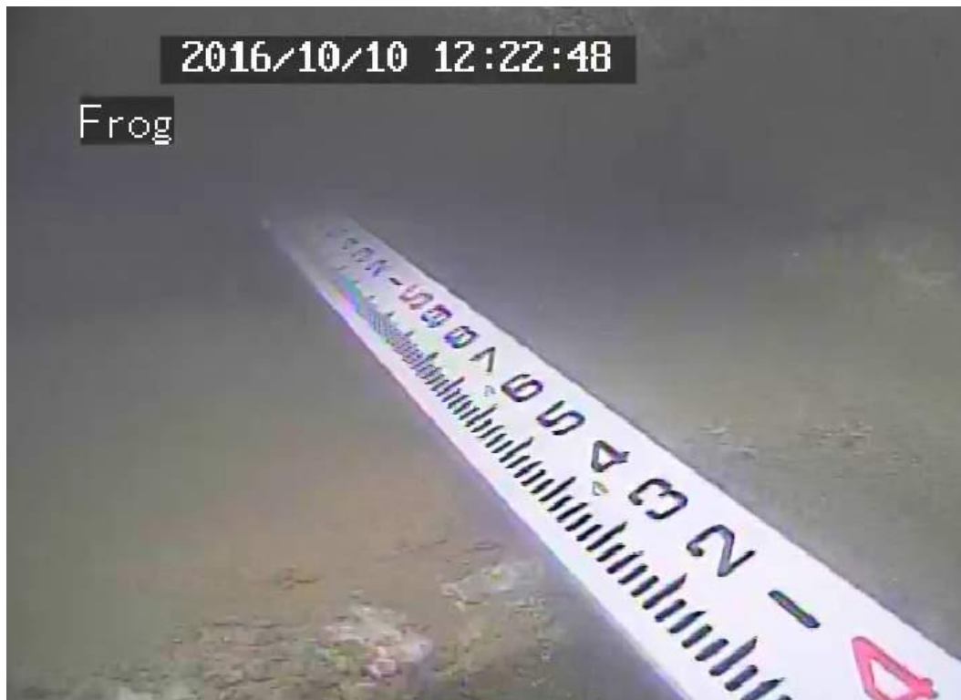
Photo 13 – Typical Downstream Scour under the Dam Toe (Approximately 1.0 feet)
